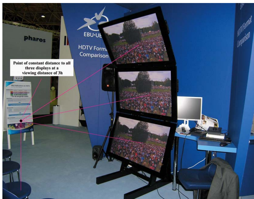
Figure 1 Three display rack with constant distance for central viewing position at 3h distance
